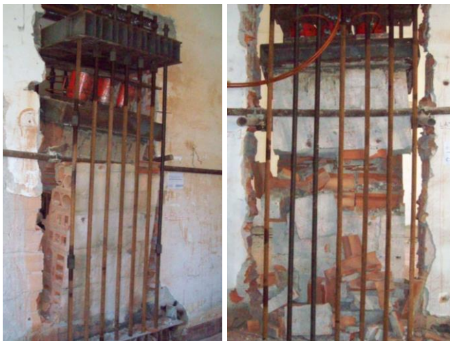
Figure 7. CS1 panel rear (a) and front (b) at the end of the test.
