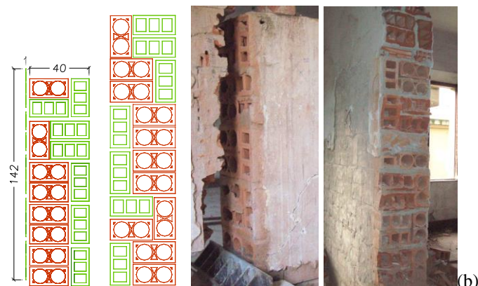
Figure 3. Graphic schemas relative to hollow brick blocks panels: examples of fronts (a) and sections (b).
